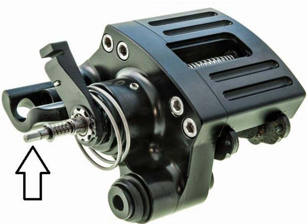
Once you have installed the calipers, carefully turn the adjuster clockwise until the brake pads touch the disc surface.
