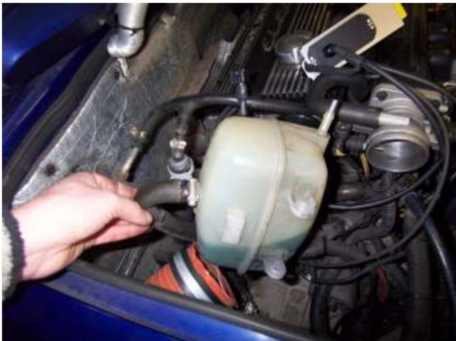
3. Undo and release the bottom hose, keep the end of the hose above the level of the engine (to avoid coolant loss) and take away the old tank. Reconnect the replacement tank from the kit to the bottom hose and re-fit it to the mount, reconnecting the small hose. Add coolant to the correct level.
