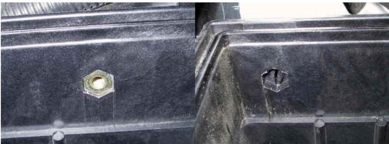
Unscrew the housing retaining bolt from the nut (left picture above) using the 10mm spanner. You probably won't be able to remove the bolt completely (due to an obstruction in the way), so leave it loosely in place.
