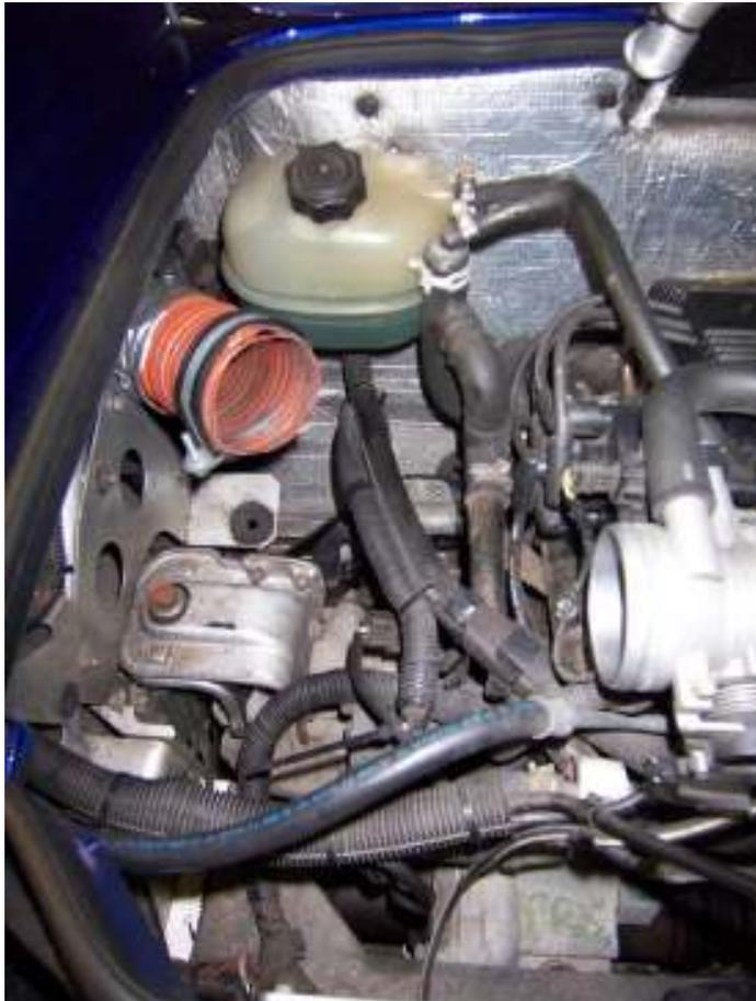
2. Undo and remove the 2 nuts and bolts (10mm heads) at the rear of the header tank
