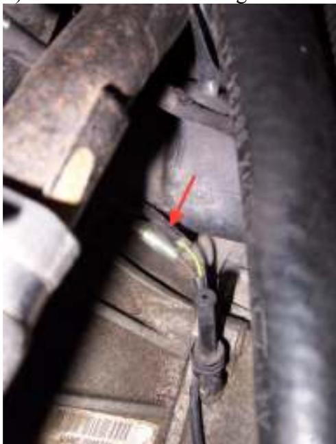
Pull the connection apart (bullet type connectors) on the **Yellow/Green** wire and re-connect with the connections from the low level kit (which has a corresponding green/yellow colour scheme):-
