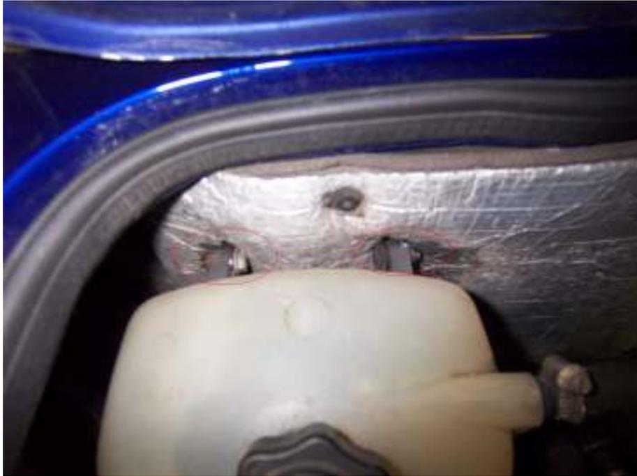
Undo and disconnect the small hose on the right of the tank. Then carefully pull the tank upwards, taking care to avoid spilling coolant through the right hand tank connection, until the tank is in a position to allow the bottom hose to be released (*Note: The bottom hose will be cable-tied to part of the wiring loom near to the underside of the tank – remove these to allow the hose & tank to come up to a level where it can be disconnected easily*).
