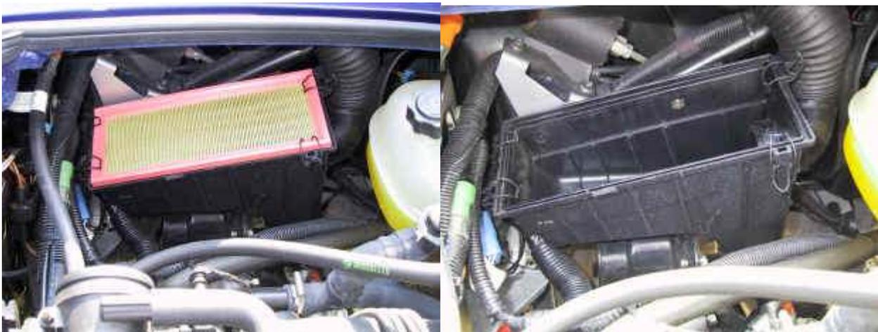
4. Removing the lower half of the air filter housing
