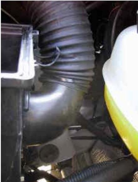
To make access easier, pull the lower air filter housing up and away from its mounts. The air intake hose is held on by a cable tie so cut this to remove.
