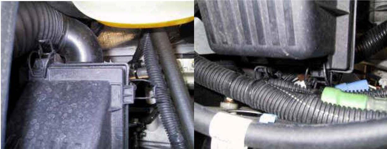
To release a fastener lift the lower part of the spring clip up towards you, releasing the fastener tension and allowing the lid to become free. Note that the clips nearest the rear of the car are difficult to get at, and the use of a screwdriver to release the left-hand one maybe necessary.
