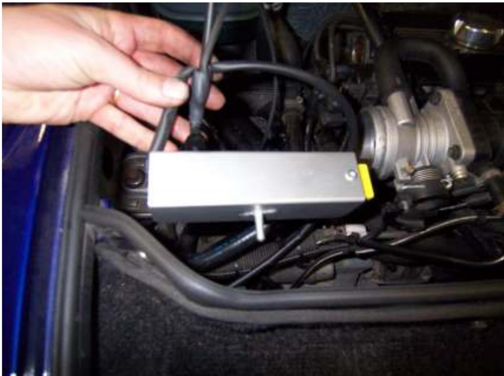
To mount drill either a 6.5 or 7mm diameter hole in approximately the following position:-
