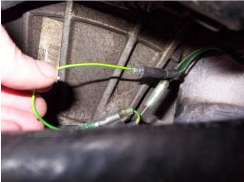
iii) The final connector is located on the far side of the multi function relay unit (MFRU), close to where the loom for the rear clam lights enters the bootbox (on post 1998 cars) – a torch will be needed to locate it:-
