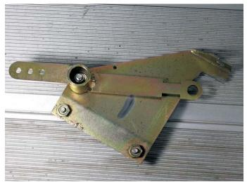
Now position the new throttle linkage over the stud/bolt. (view the picture to see the correct position of the throttle linkage)
