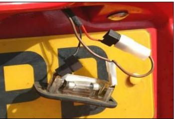
Unscrew and drop down the right hand number plate light as shown.
