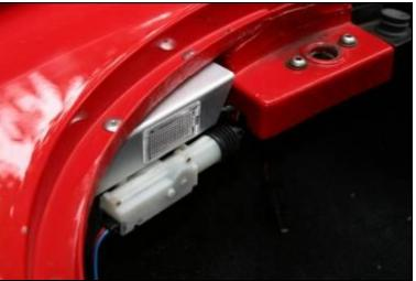
Once the complete unit is installed, put a dab of silicon in the rivet centres to alleviate water ingress into the boot area.
