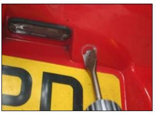
Mark and drill a small pilot hole with the drill provided to the dimensions as shown, then use the 19mm drill bit provided & carefully drill a full size hole as shown. Be careful to slow just before you go completely through as there may be wires behind.
