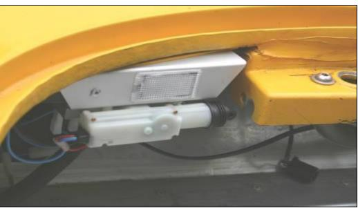
Drill out the two pop rivets using the 4.2mm drill piece provided.
