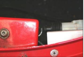
Connect the U shaped cable connector exactly as shown above and tighten with the 2mm Allen key provided. You will need to put your head into the boot "upside down" for a few seconds to see where to attach. Using the file provided, shape a semi circular slot as in picture for the solenoid connector rod to pass through.
