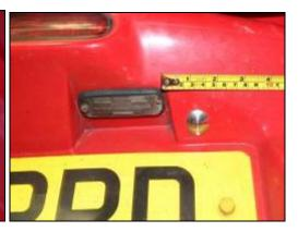
Thread the two black wires through the 19mm hole. MAKE SURE THE 19MM NUT IS ON THE CABLE PRIOR TO PUSHING THROUGH THE HOLE. Screw the 2 black wires to the stainless steel switch then locate & tighten the switch into place as shown.
