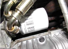
Connect the new braided hoses to the oil cooler unit as shown in top picture ,the short braided hose fits to the Right hand side of the cooler and the longer hose fits to the Left hand side.
