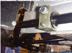
Use plenty of the Molybdenum grease supplied around the bar and the nylatron bushes. Loosely fit the bushes to the bar and offer up into place making sure you have the bushes the correct way around (M5 bolt head is recessed to the chassis) and the right way up (M10 bolt/sleeve to the top). Once satisfied gently tighten the M5 nut and fit the M10 long bolt through the sleeve and torque to 35lb pr ft.
