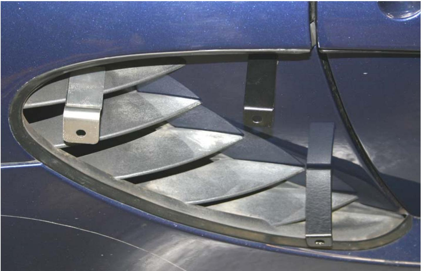
Mark the vehicles side panel through the two "U" shaped brackets in the centre hole (middle of the 5 holes).
