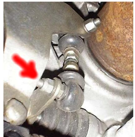
7. Remove the old rod ends from the bell-crank, and then dis-assemble them from each other. Make up the new rod ends to mimic the old ones, setting them distance from the centres to the same as the old ones (this should be about 70mm). Then bolt one end back to the bell-crank as shown.
