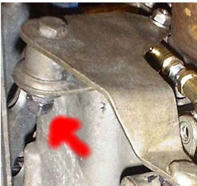
6. Remove the bell-crank nuts (shown left), this is a Nyloc and half nut. When removed, the bell-crank should be slid off with the old joints attached.
