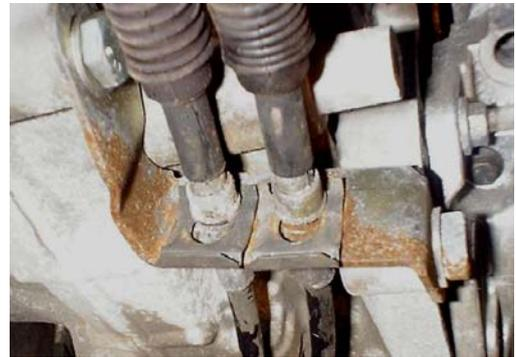
4. Push out the old rubber bushes from the ends of the gear cables, then, move the cable out of the way.
