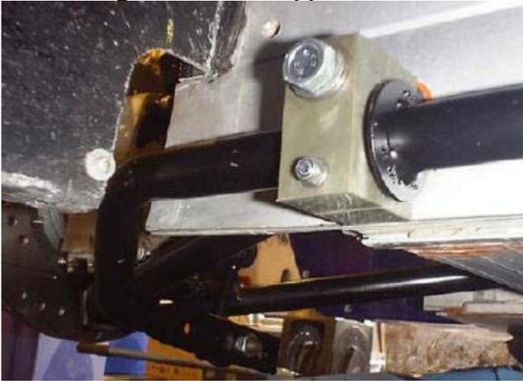
Use plenty of the Molybdenum grease supplied around the bar and the nylatron bushes.
