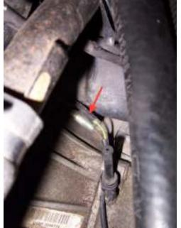
Pull the connection apart (bullet type connectors) on the *Yellow/Green* wire and re-connect with the connections from the low level kit (which has a corresponding green/yellow colour scheme):-
