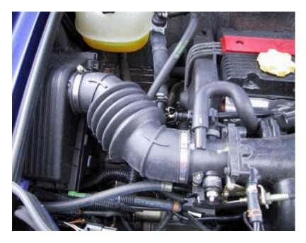
*Note*: The clip at the throttle body end may not be a jubilee clip. If it is as shown below, a flat bladed screwdriver is required to spring it apart.
