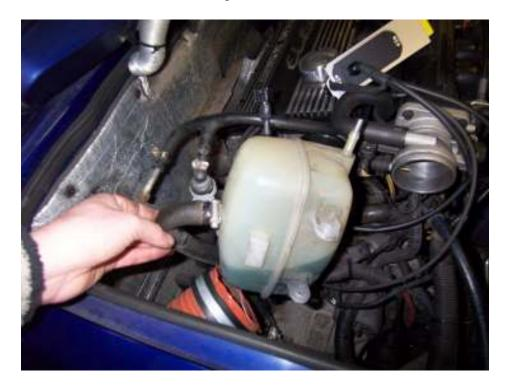
3. Undo and release the bottom hose, keep the end of the hose above the level of the engine (to avoid coolant loss) and take away the old tank. Reconnect the replacement tank from the kit to the bottom hose and re-fit it to the mount, reconnecting the small hose. Add coolant to the correct level.
