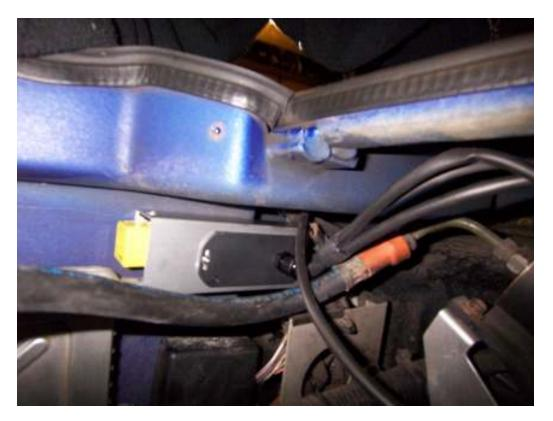
Finally, find a sensible routing for the wires and secure with cable ties, before refitting the air filter housing or induction kit:-
