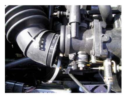
2. Release the 4 spring clip fasteners that hold the air filter housing top to the lower half:-
