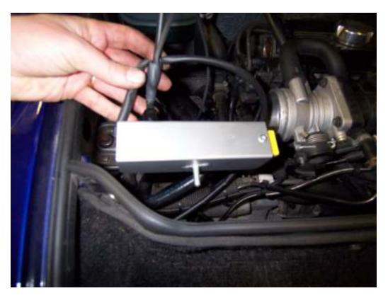
To mount drill either a 6.5 or 7mm diameter hole in approximately the following position:-
