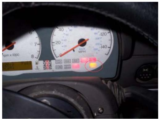
Note: This will stay illuminated for approximately 15 seconds after the circular 'float' ring is released (and thus returns to the top of the coolant in the tank).
