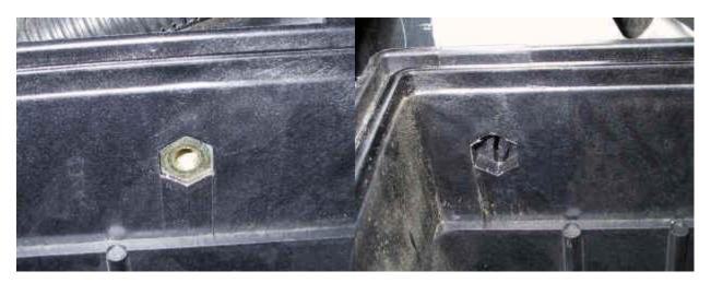
Unscrew the housing retaining bolt from the nut (left picture above) using the 10mm spanner. You probably won't be able to remove the bolt completely (due to an obstruction in the way), so leave it loosely in place.
