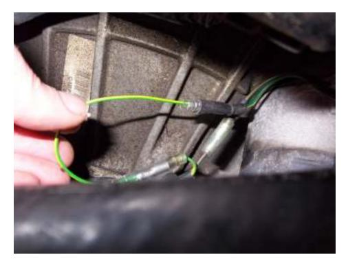
iii) The final connector is located on the far side of the multi function relay unit (MFRU), close to where the loom for the rear clam lights enters the bootbox (on post 1998 cars) – a torch will be needed to locate it:-
