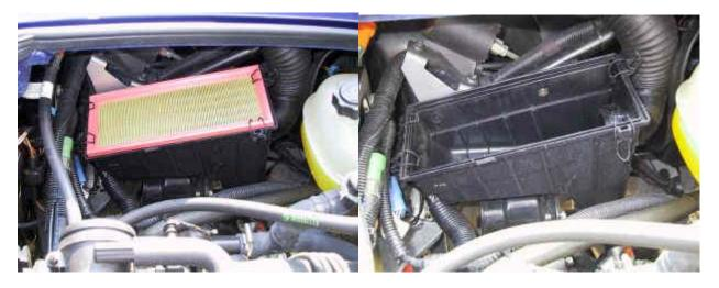
4. Removing the lower half of the air filter housing
