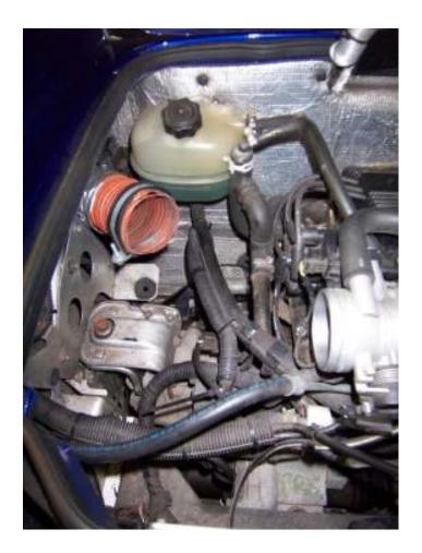
2. Undo and remove the 2 nuts and bolts (10mm heads) at the rear of the header tank
