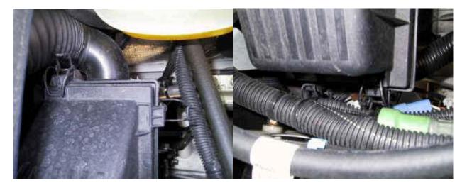
To release a fastener lift the lower part of the spring clip up towards you, releasing the fastener tension and allowing the lid to become free. Note that the clips nearest the rear of the car are difficult to get at, and the use of a screwdriver to release the left-hand one maybe necessary.
