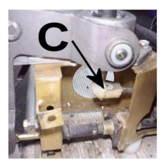
Remove lever from the base unit leaving the top half of the plastic cup in place.
